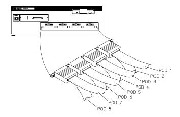
Use this table to connect cables from the Agilent Technologies 16601A logic analyzer to the connectors in the target system.
