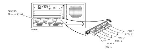
Use this table to connect cables from the Agilent Technologies 16550A logic analyzer to the connectors in the target system.
