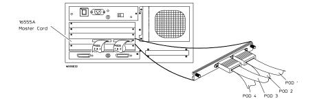
Use this table to connect cables from the one-card Agilent Technologies 16554/55/56/57 logic analyzer to the connectors in the target system.
