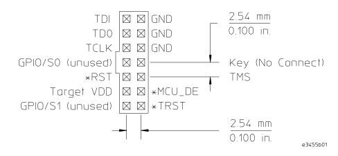
**NOTE:** MCU\_DE, RST, and all of the JTAG signals except TDO require a 10K pull-up resistor for deterministic operation in the absence of an emulation module.
