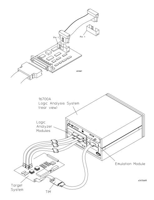
**7** Turn on the power to the logic analysis system and then the target system.
