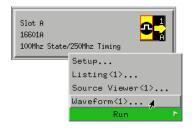
You can also use the Waveform display in the state analysis mode to display state timing diagrams.
